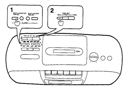
Press and hold the alarm 1 (or 2) display/adjust button.
