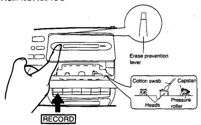
The head assembly, capstan and pressure roller are in constant contact with the tape. If these parts are dirty, the sound quality will be impaired. Periodically, clean these parts as shown.
