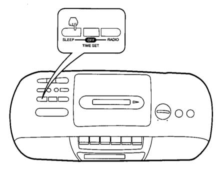
You can set the clock radio to play up to about 59 minutes, the shut off automatically.
