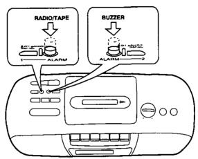
The buzzer alarm and the radio (or tape alarm) are set at the same time. Both alarms will activate simultaneously.
